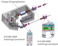
Figure 5: The layout of Folding Segment 1 and required matching cryomodules.
