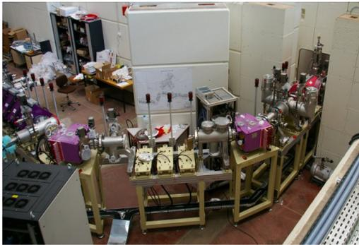
Figure 3: The light ion LEBT2 line installed at CEA IRFU/Saclay.
