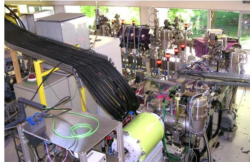
Figure 4: The heavy ion ECR source and LEBT1 line installed at LPSC/Grenoble
