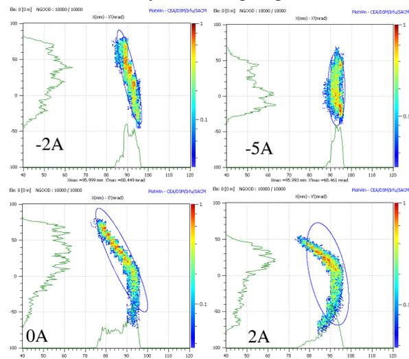
Figure 5: Effect of the hexapole tuning on the horizontal emittance ( $^{16}O^{6+}$ , 32kV, March 2010).
