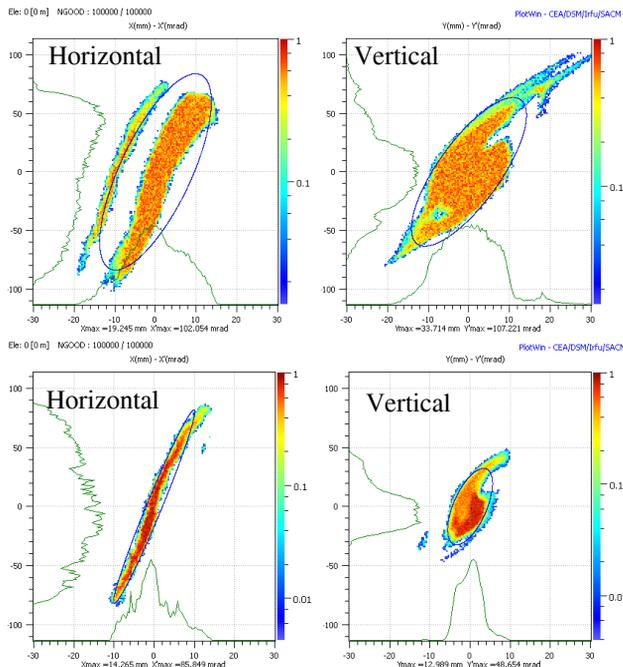
Figure 7: Test of the separation power with Xe at 40kV (up) slits fully opened:  $^{132}\text{Xe}^{25+}$  &  $^{16}\text{O}^{3+}$  are visible; (bottom) slits opened at  $\pm 5\text{mm}$ , only  $^{132}\text{Xe}^{25+}$  remains.
