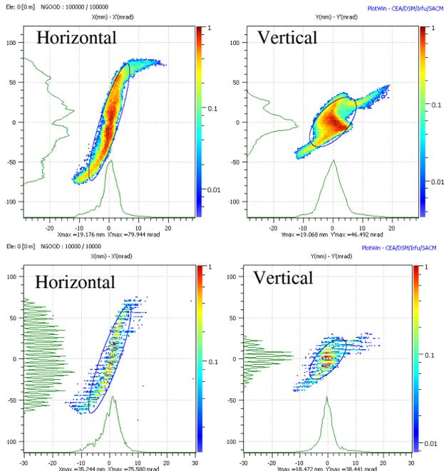
Figure 6: Emittance measurements in CW (up) and pulsed (bottom) source mode ( $^{40}\text{Ar}^{12+}$ , 40kV, June 2010).
