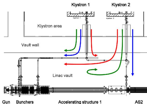
Figure 2: The new waveguide configuration.
