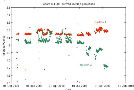
Figure 1: Perveance record of klystrons through 2009.
