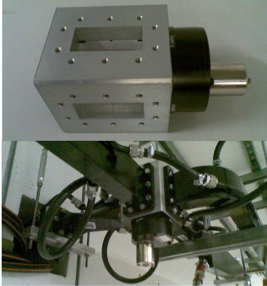
Figure 3: WR284 waveguide switch (above) and switch assembly in situ (below).
