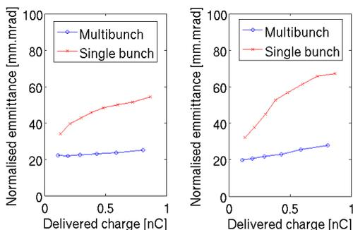
Figure 5: Beam emittance as a function of charge for single klystron operation: horizontal emittance on left, vertical emittance on right.
