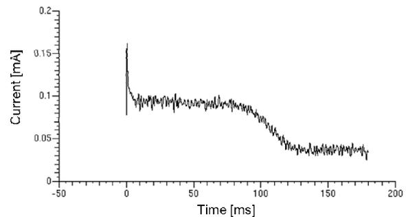
Figure 4: Beam current in the booster.
