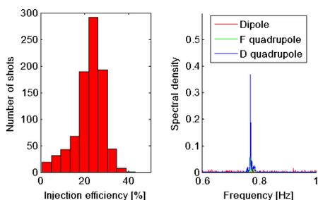
Figure 6: Injection efficiency and magnet stability.
