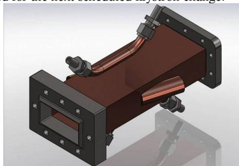
Figure 7: Design for a new arc detector viewport.
