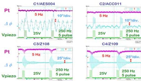
Figure 16: Mechanical vibration mode of four FNAL/DESY cavities by 5 continuous pulses of Piezo.
