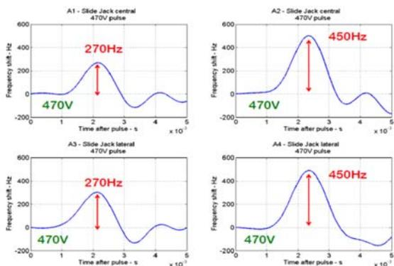
Figure 15: Single pulse response of four KEK cavities by Piezo tuner.
