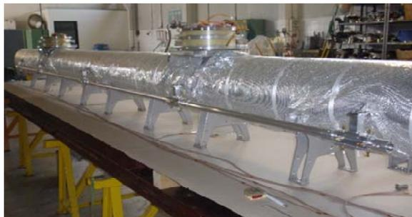
Figure 4: Completed gas return pipe and support posts for Module-C in the company of Italy.
