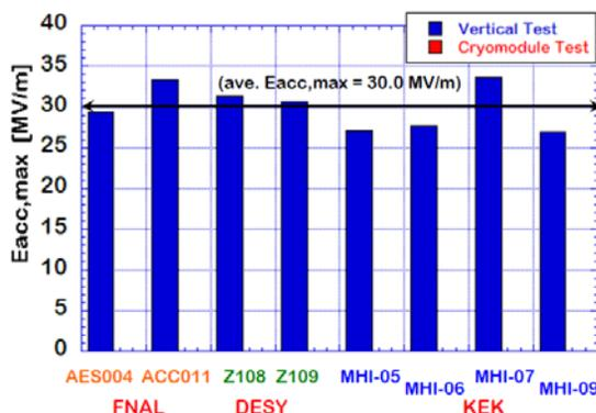
Figure 5: Field gradients of 8 cavities for the S1-Global cryomodule.
