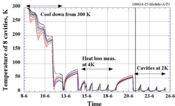
Figure 14: First cool-down of 8 cavities in S1-G cryomodule from June 8 to June 26.
