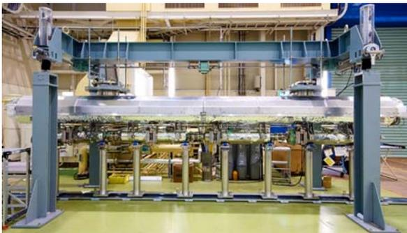
Figure 11: Four KEK cavity string supported from gas return pipe.
