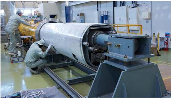
Figure 10: Inserting the Module-C cold mass into cryostat.
