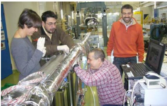
Figure 8: Mounting tuners on DESY/FNAL cavities by the INFN/FNAL team.
