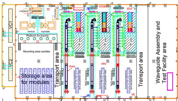
Figure 6: DESY's Accelerator Module Test Facility (AMTF).
