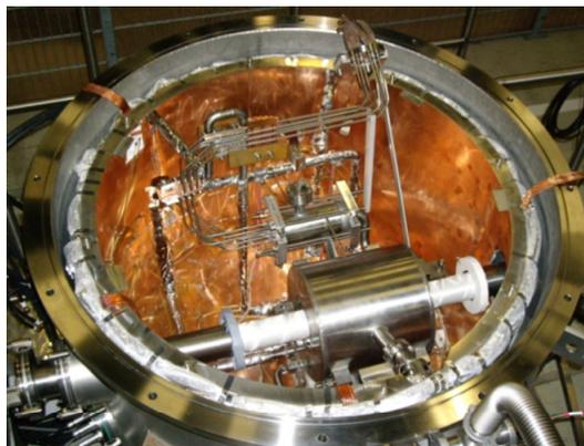
Figure 7: Cold quadrupole magnet produced by CIEMAT, in DESY's test cryostat.
