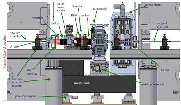
Figure 9: Intersection between two adjacent undulators.
