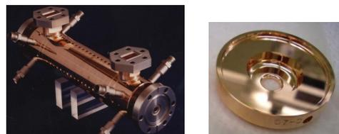
Figure 2: CERN made 30cm X-band accelerator structure.
