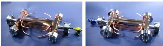
Figure 5: Prototype twin structures of T18. Left is for test at KEK and right for test at SLAC.
