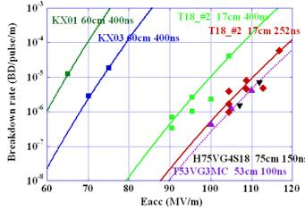
Figure 9: Breakdown rates of 53cm undamped structure, 60~75cm HDDS structures and undamped 20cm CLIC prototype structures, T18.
