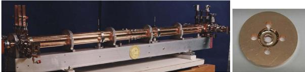
Figure 3: 1.8m RDDS1 structure and constituent cell.
