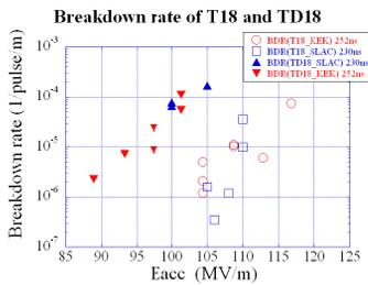
Figure 10: Breakdown rates of twin TD18's.
