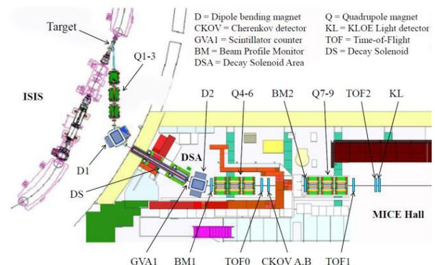
Figure 1: The MICE beam-line at ISIS [3].
