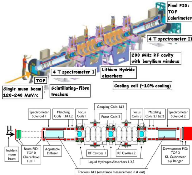
Figure 2: The MICE Cooling Channel: top, 3D cutaway view; bottom, 2D view.
