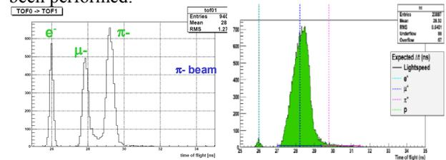
Figure 4: Time-of-flight (TOF) distributions for particles in (left) a pion beam and (right) a muon beam with a large energy spread (data taken Dec. 2009).
