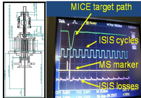
Figure 5: Left, target-assembly schematic diagram; right, on-line monitoring display of target operation.
