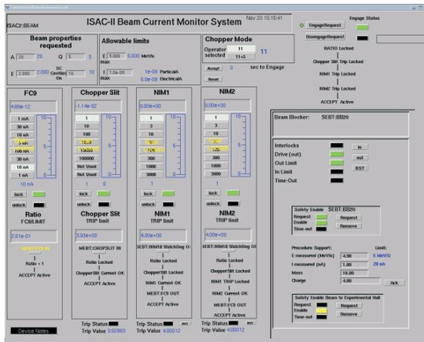
Figure 6: The EPICS CMS interface displays beam parameters (top left), license allowable limit, chopper operational mode, monitor read backs and trip limits.
