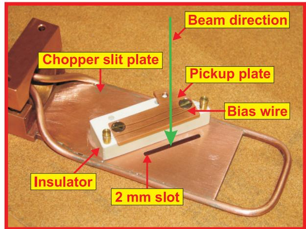
Figure 3: The upgraded chopper slit. The main bunch goes through the 2 mm slot while the satellites land on the pick up plate.
