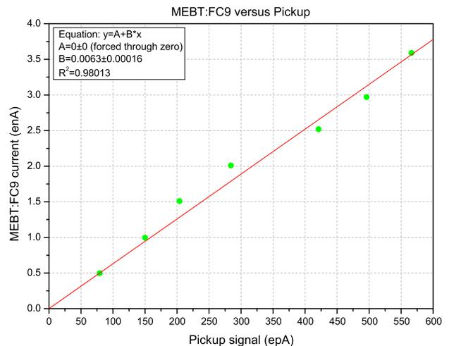
Figure 4: A test of the linearity of the chopper slit pickup.
