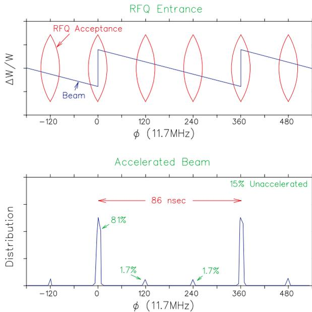
Figure 2: Time structure of the beam at the exit of the RFQ. The main peak frequency is 11.78 MHz. The satellites are a result of the 35.36 MHz RF.
