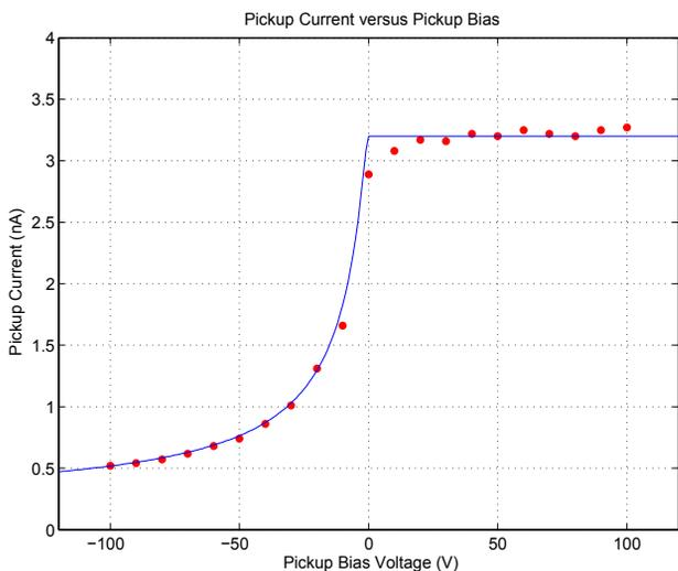
Figure 5: The effect on the signal of the bias voltage.
