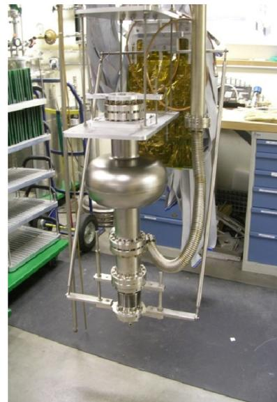
Figure 2: The 805 MHz cavity with a moveable coupler and a vacuum line attached at the bottom.
