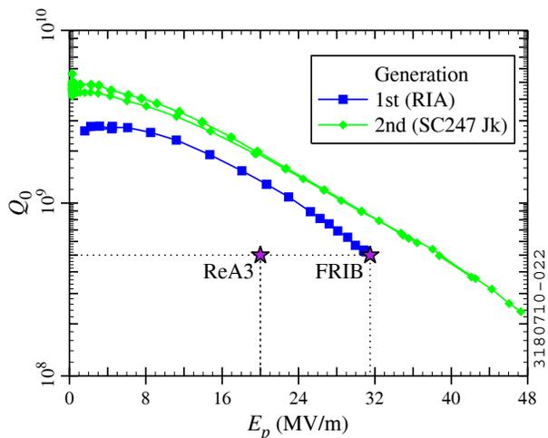
Figure 3: Dewar test results at  $T = 4.3$  K for first-generation and second-generation  $\beta_m = 0.085$  QWRs.
