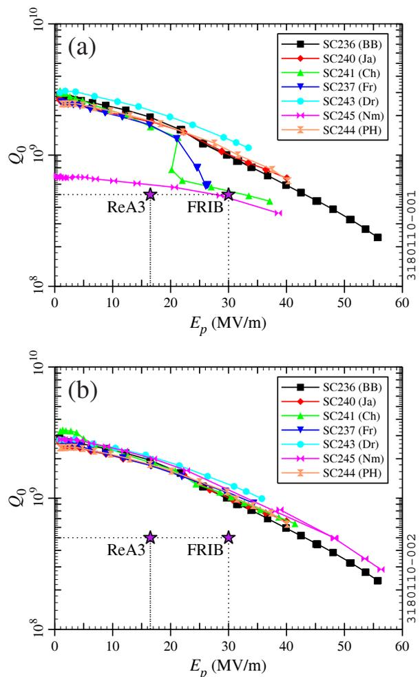
Figure 2: Dewar test results at  $T = 4.3$  K for  $\beta_m = 0.041$  QWRs: (a) measurements with no cooling of the bottom flange; (b) measurements with cooling of the bottom flange for all resonators except the first one.
