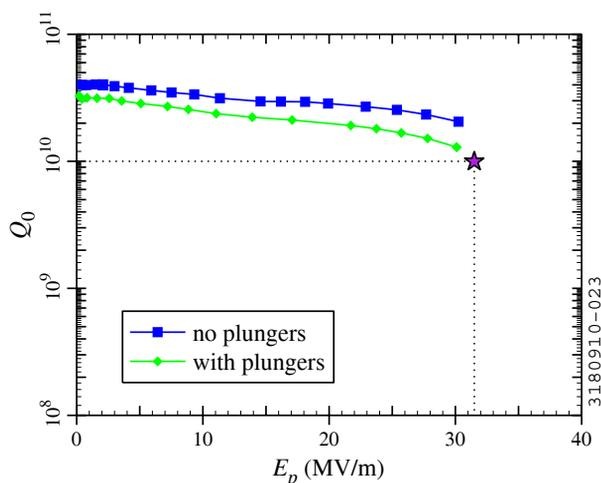
Figure 4: Dewar test results at  $T = 2$  K for the first prototype  $\beta_m = 0.53$  HWR.
