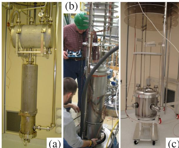
Figure 1: Resonator photographs: (a)  $\beta_m = 0.041$  QWR with helium vessel in clean room; (b)  $\beta_m = 0.085$  QWR without full helium vessel being lowered in to the Dewar; (c)  $\beta_m = 0.53$  HWR in the clean room.
