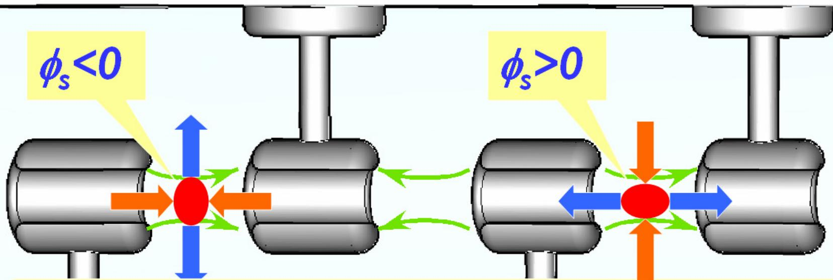
**Both stability of motion is obtained just with the rf acceleration field!**
