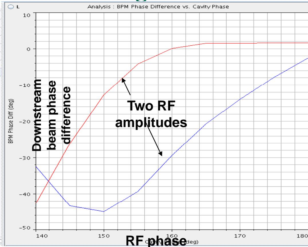
Downstream beam behavior has complicated dependence on RF phase and amplitude – each cavity has a unique signature
