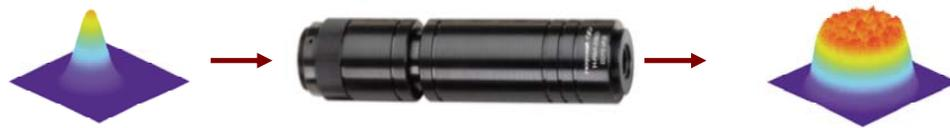
Gauss to flat top transformation using a commercial aspheric lens (Newport Corp)
