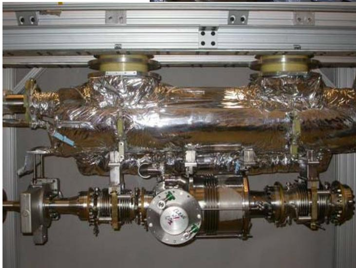
Cavity string before installation into cryomodule
