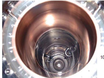
**352 MHz SOLEIL cavity based on the LEP cavity technology, Nb-Cu.**
