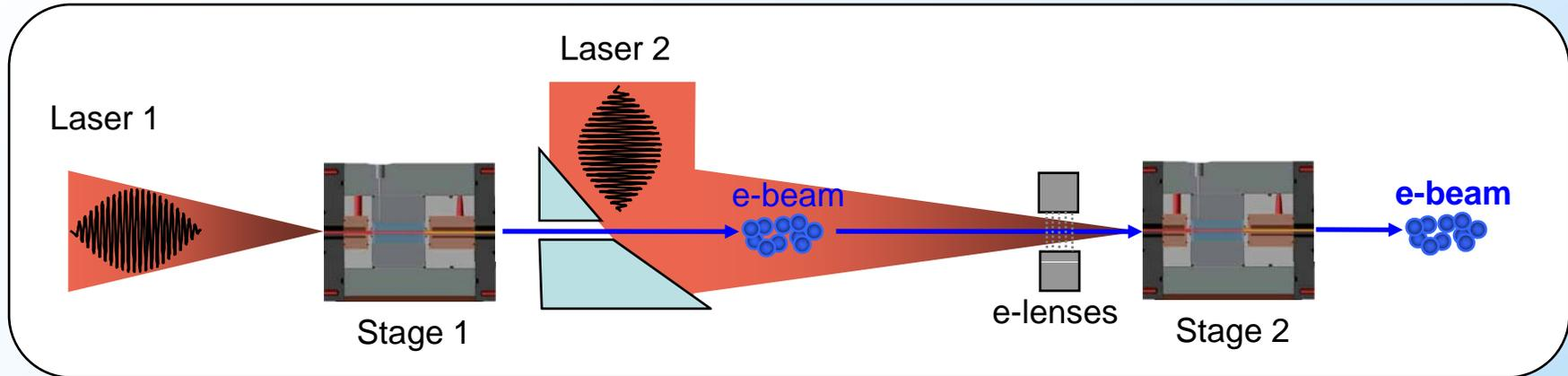
Minimum distance between the stages is limited by mirror breakdown ( $\sim 10\text{m}$ )
