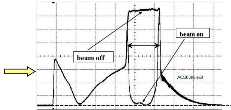
RF power at output of accelerating structure
