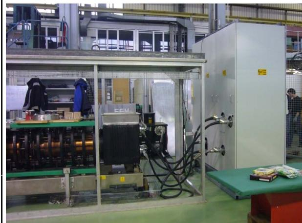
**352 MHz klystron pulsed test**
