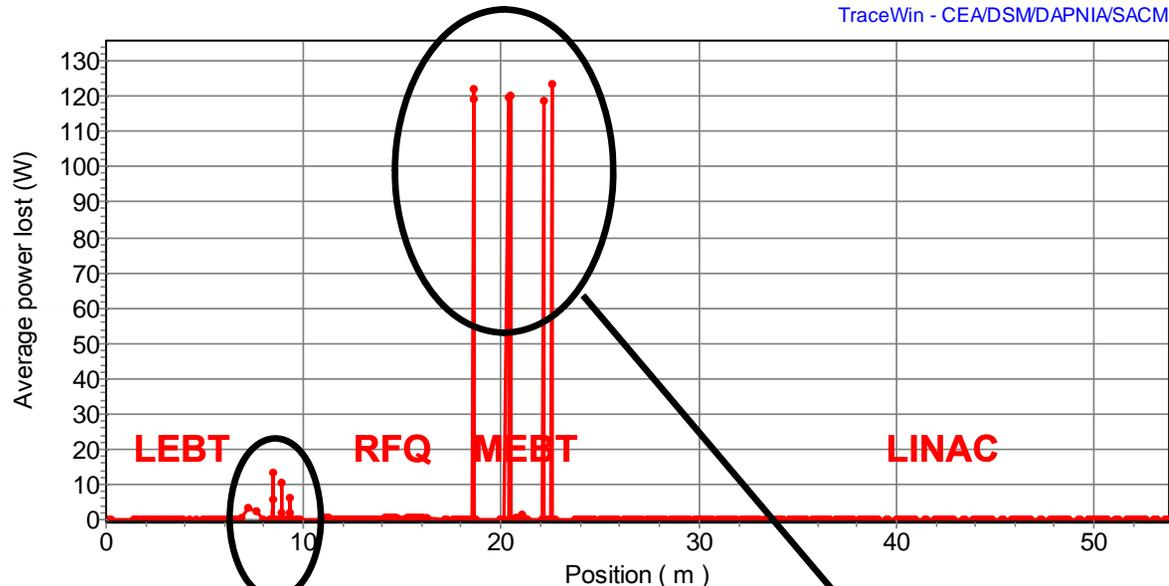
6 slits system to remove beam halo coming from the RFQ in order to protect the linac.
