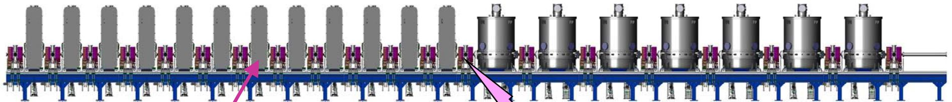
Each cryomodule is installed on independent supports with alignment adjustments
