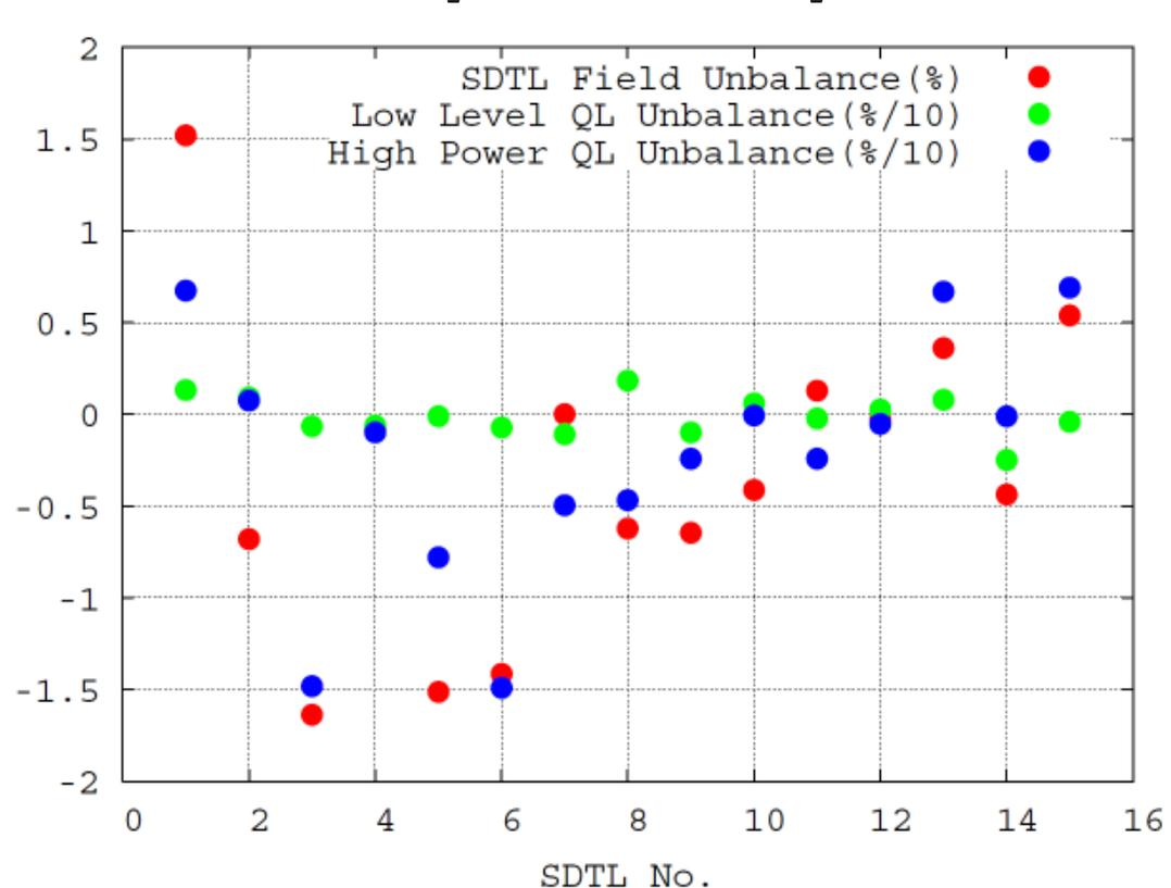
RF-Fields of SDTL03A&B (Max. Unbal. due to 28mA & 100μs Beam Loading :Unexpectedly Large Unbal.) and SDTL12A&B (Min.Unbal.)
