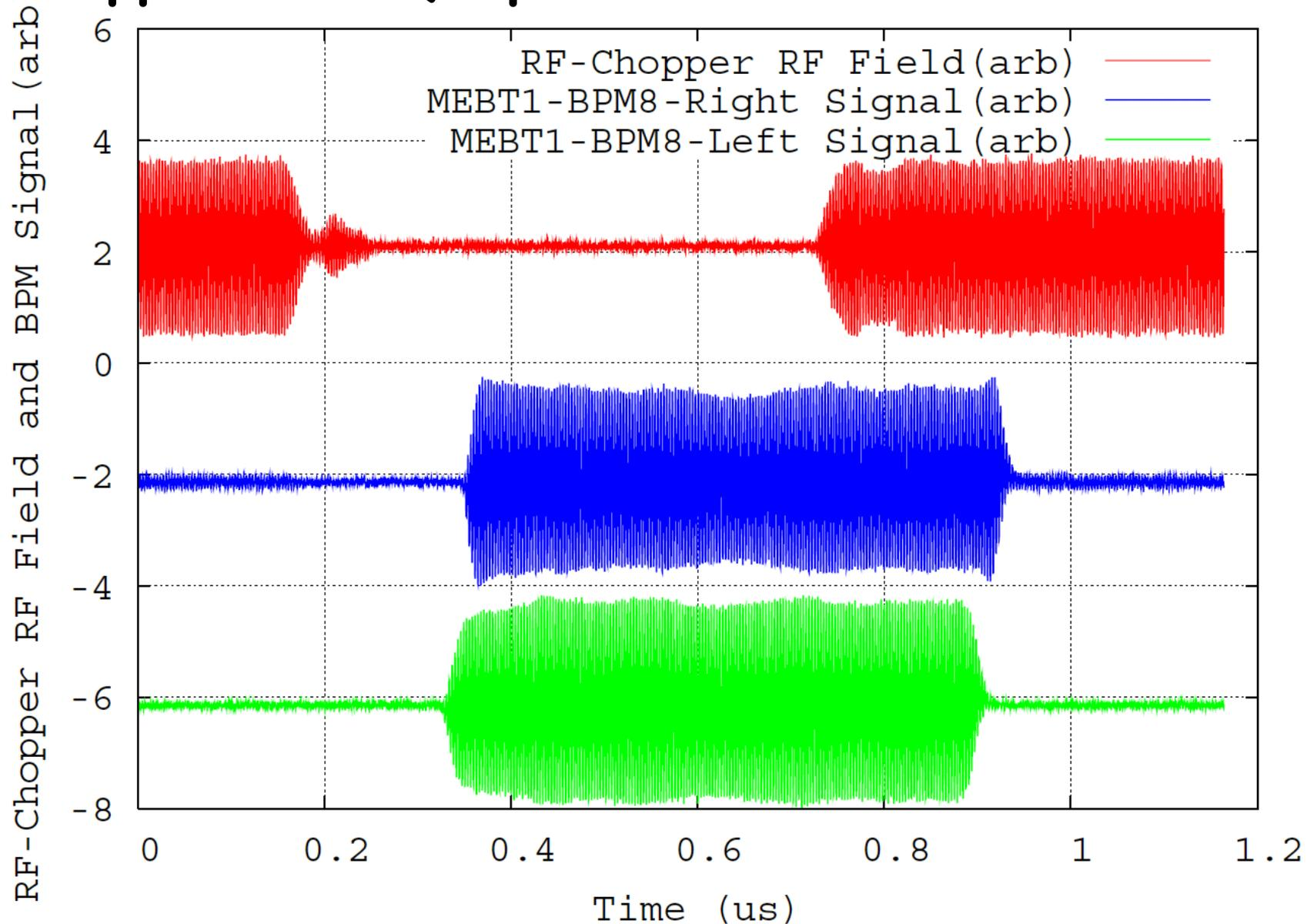
**Ring**ing of RF-field of RF-Chopper at **RF on/off** Transient-Time
