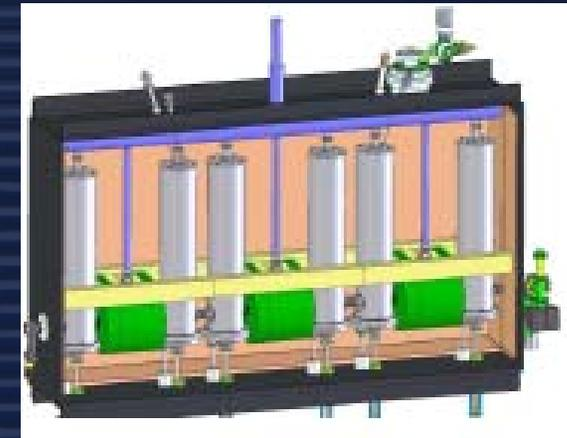
2<sup>nd</sup> cryomodule housing 6 QWRs with beta 0.041
