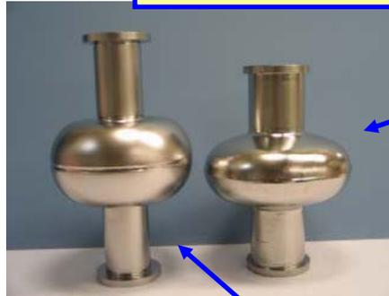
Tesla-shape cavity for comparison
