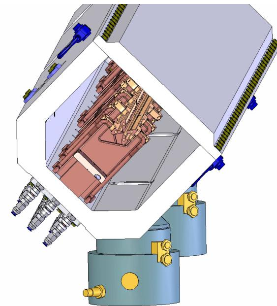
Al-cavity, st.steel flanges, block milling, cooling tubes (el,st),
