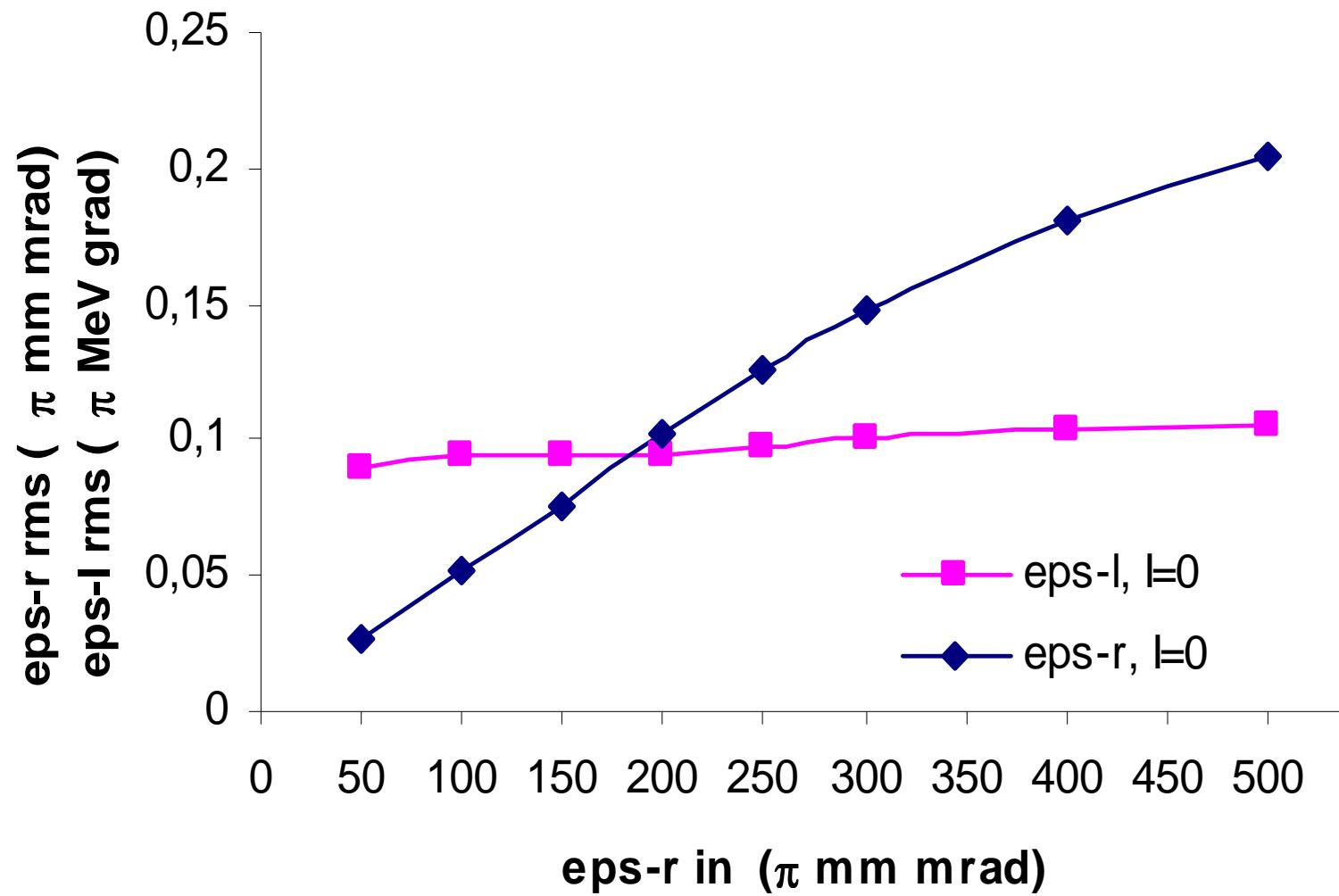
radial and longitudinal output emittance as function of input emittance
