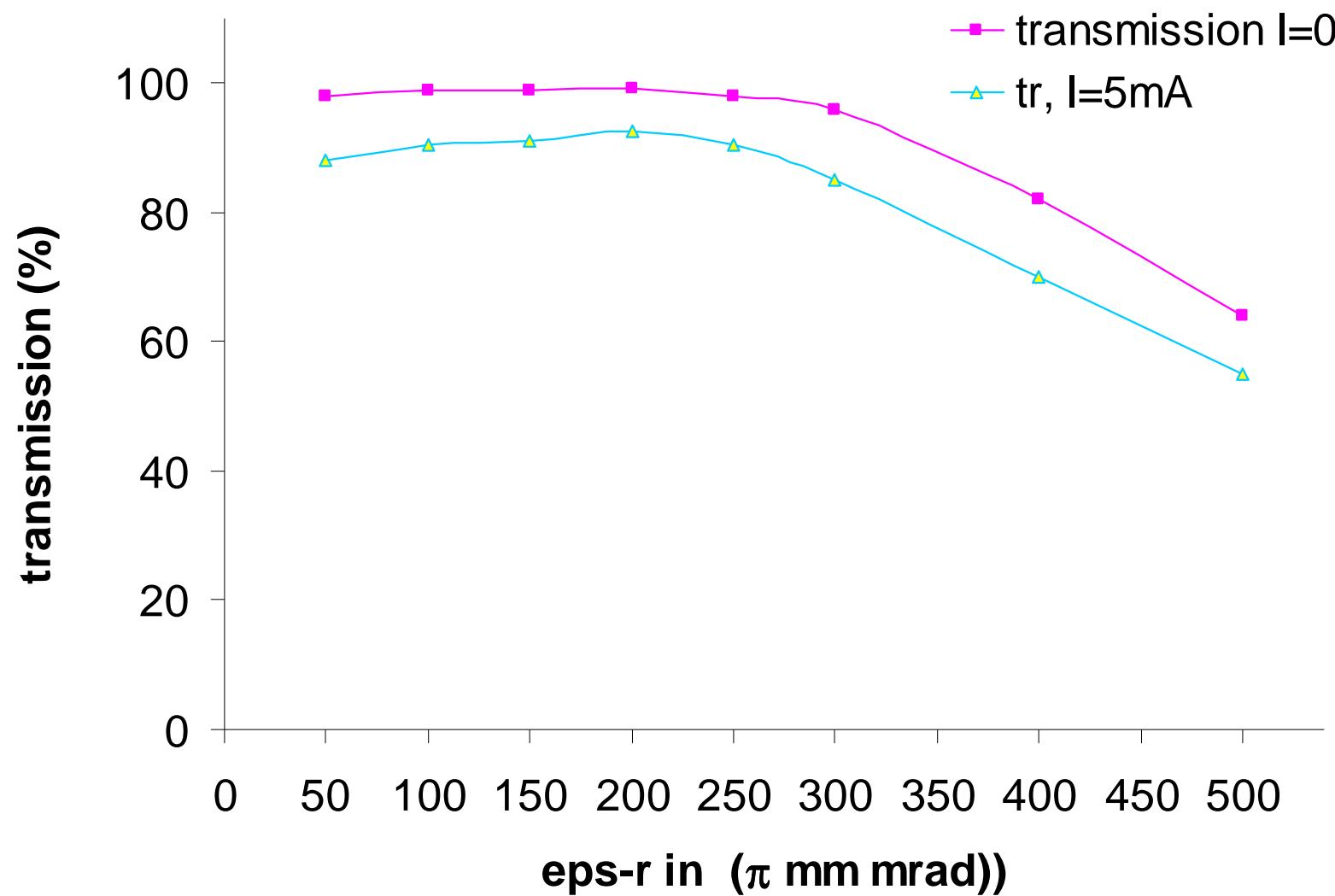
**Transmission as function of the input emittance**
