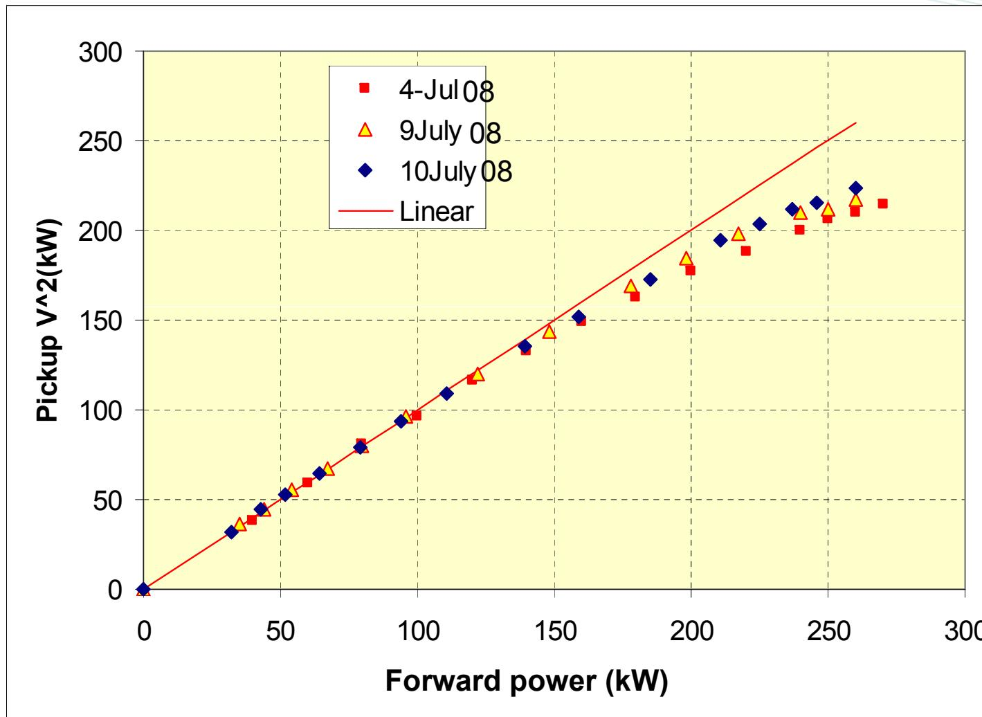
Parting from the linear relation indicates onset of dark current due to poor conditioning
