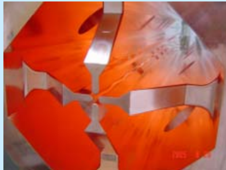
Four vane structure RFQ
