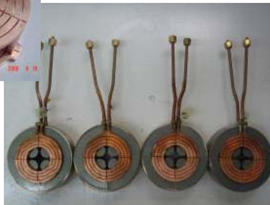
J-PARC type electromagnetic quadrupoles
