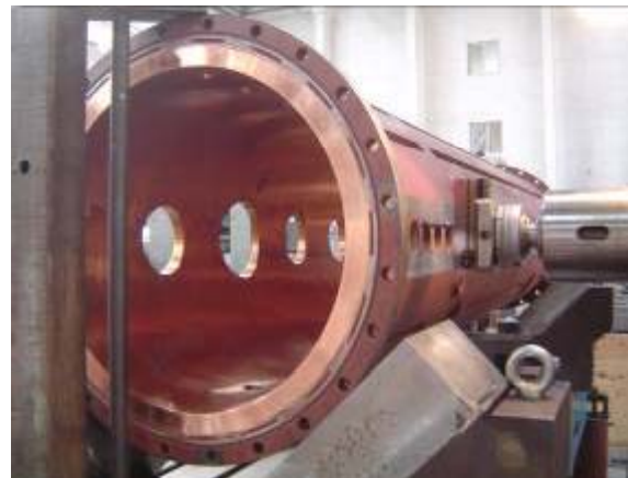
DTL tank under final machining of the drift tube holes
