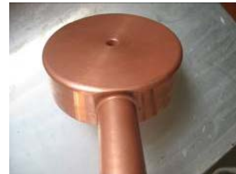
Bulk copper for drift tube by EBW
