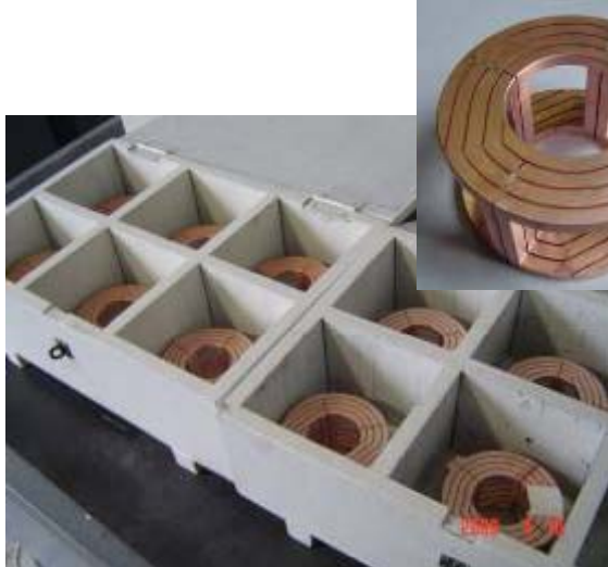
J-PARC type electromagnetic quadrupoles
