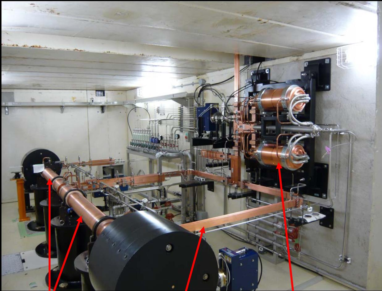
Accel. struct. Waveguide RF pulse compressor
