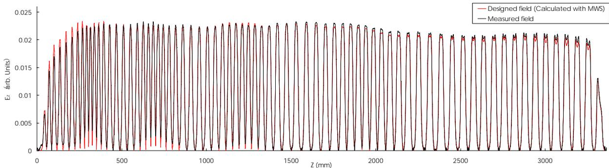
Figure 7: Electric field along the beam axis as functions of the beam coordinate,  $Z$  for the APF IH-DTL. The black and red curves show the measured and designed electric field, respectively. The designed field was calculated with MWS.
