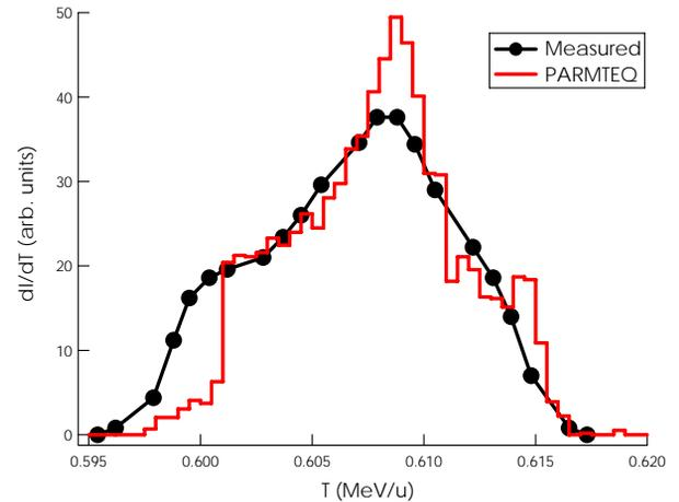
Figure 10: Kinetic energy distributions of a carbon beam from the RFQ linac. The filled dots and histogram show the results of the measurement and a PARMTEQ calculation, respectively.
