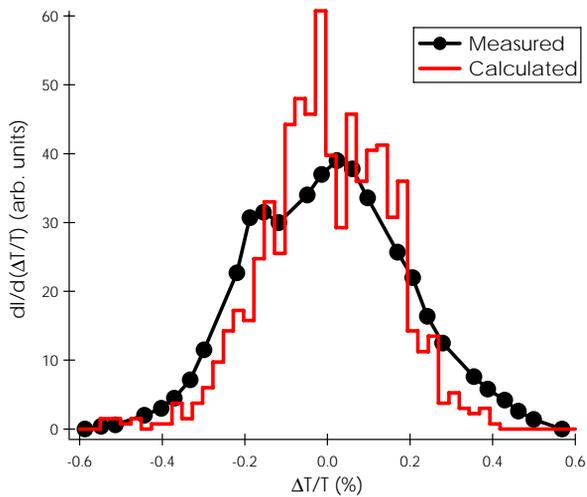
Figure 12:  $\Delta T/T$  distributions of a carbon beam from the APF-IH-DTL. The filled dots and histogram show the result of the measurement and a tracking simulation, respectively.
