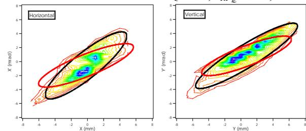
Figure 11: Contour plots show the horizontal and vertical phase-space distribution of a carbon beam from the APF IH-DTL (see text).
