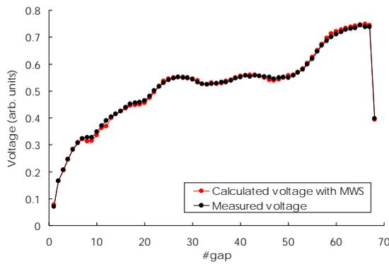
Figure 5: Gap voltages along the beam axis as functions of the gap number for the model cavity. The black and red dots show the measured and calculated gap-voltages, respectively.
