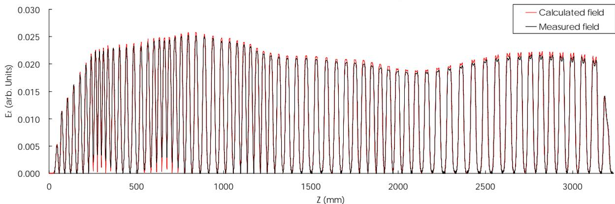
Figure 4: Electric field along the beam axis as functions of the  $Z$  of the beam coordinate,  $Z$ , for the model cavity. The black and red curves show the measured and calculated electric field with MWS, respectively.
