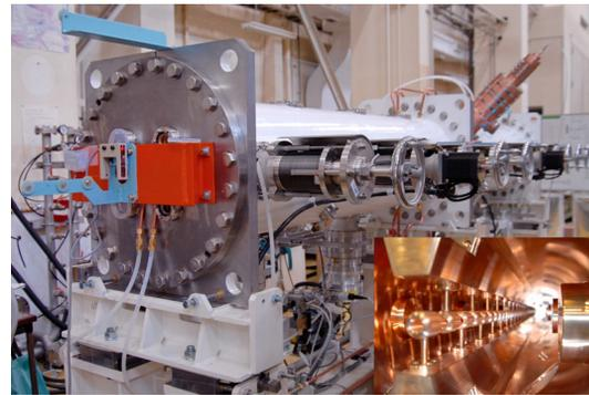
Figure 6: A picture of the APF IH-DTL during turning of the electric-field distribution in the cavity.
