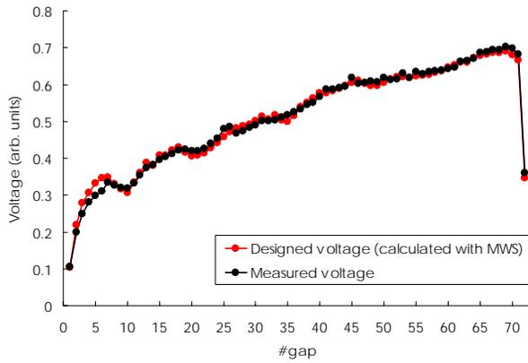
Figure 8: Gap voltages along the beam axis as functions of the gap number for the APF IH-DTL. The black and red dots show the measured and designed voltage, respectively.
