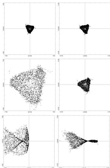
Figure 9: Beam profile (left) and momentum space (right) from CAPRICE with 1.0 T flux density hexapole, after extraction (first row), behind a focusing solenoid (second row), and after  $m/q$  separation (third row).
