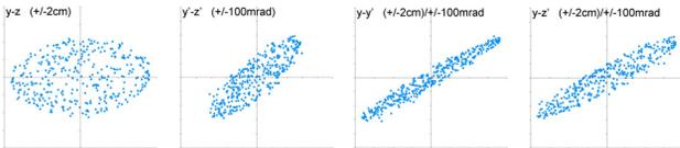
Figure 3: Different projections of the 6D phase space for the beam extracted from ARC-ECRIS: real space, momentum space, emittance, and a mixed phase space. In this solution, space charge effects are still neglected.
