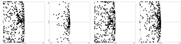
Figure 10: Expected beam cross sections behind the dipole for different magnetic settings of MG-ECRIS.
