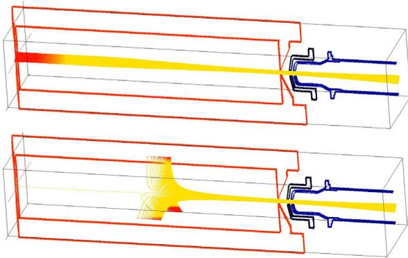
Figure 4: Magnetic field lines for different coil settings of the MS-ECRIS. Top: design value, middle coil switched off. Bottom: design values, injection field decreased to 60%. The red part of the field line indicates that the value of flux density is above that value at extraction aperture.
