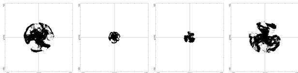
Figure 8: Beam cross sections from SUPERNANOGAN behind the beam line solenoid with increasing magnetic focusing strength from left to right.
