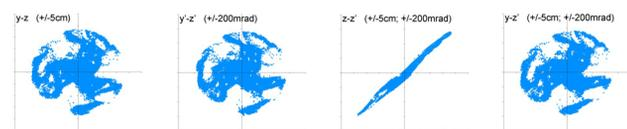
Figure 1: Different projections of the 6D phase space from left to right: beam cross section, momentum space, emittance, mixed phase space. Total current for the simulation 3 mA, shown is one charge state only.
