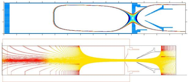
Figure 6: Magnetic field lines and magnetic flux density for the SECRAL ion source.
