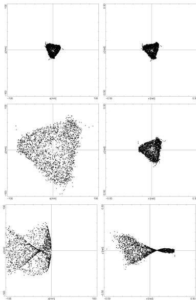
Figure 9: Beam profile (left) and momentum space (right) from CAPRICE with 1.0 T flux density hexapole, after extraction (first row), behind a focusing solenoid (second row), and after  $m/q$  separation (third row).
