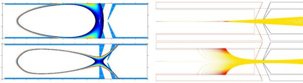
Figure 2: Magnetic structure of the arc-ecris: lines of constant  $|\vec{B}|$  and magnetic field lines in horizontal and in vertical projection.
