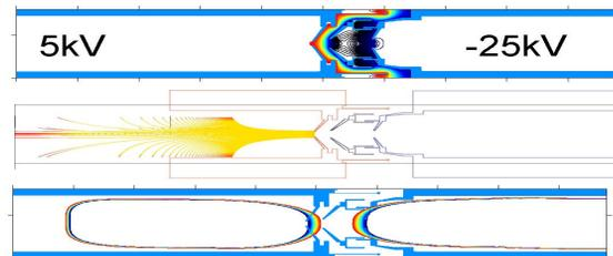
Figure 7: Superconducting ECRIS from Riken: top: electric potential, middle: magnetic field lines, bottom: lines of constant  $|\vec{B}|$ .
