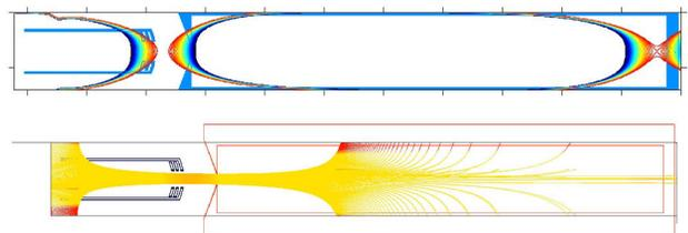
Figure 5: Hybrid source: superconducting mirror coils and permanent magnets for the hexapole.
