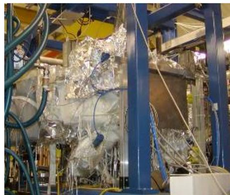
Figure 2: Photoinjector wrapped in heating blankets for a bakeout that resulted in an excellent pre-test vacuum.
