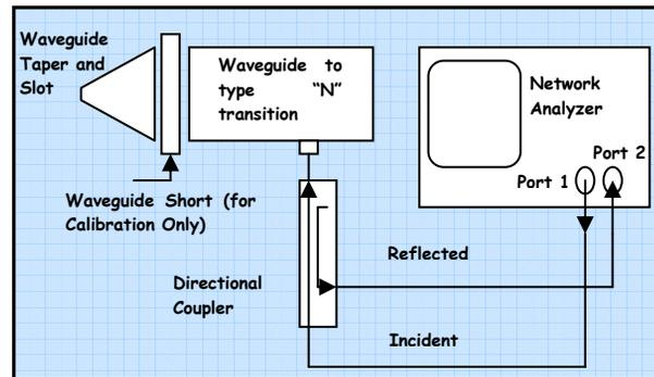
Figure 4: Calibration and coupling measurement for the waveguide couplers.
