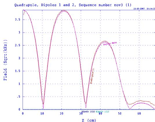
Figure 3: Comparison of the bead-pull measurement with the field distribution from Superfish. The agreement is better than 7%.
