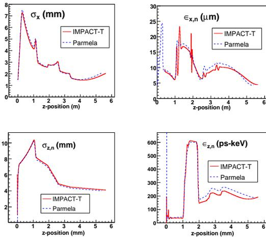
Figure 2: Beam moments as a function of the distance from the cathode. The average beam current is 750 mA and the radius of the beam at cathode is 3 mm.
