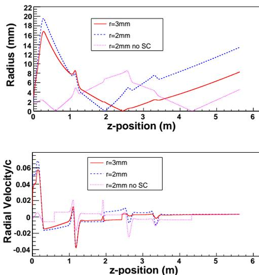
Figure 5: Top plot: the distance between the outermost particle and the beam axis as a function of the distance from cathode, when the initial beam radius was 2 mm, 3 mm, and 2 mm with space charge calculation turned off. Bottom plot: the radial velocity of the outermost particle as a function of the distance from cathode.
