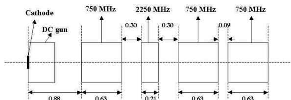
Figure 1: Schematic layout of the AES/JLab photoinjector. Emittance compensation solenoid is not shown. All dimensions are in meters.
