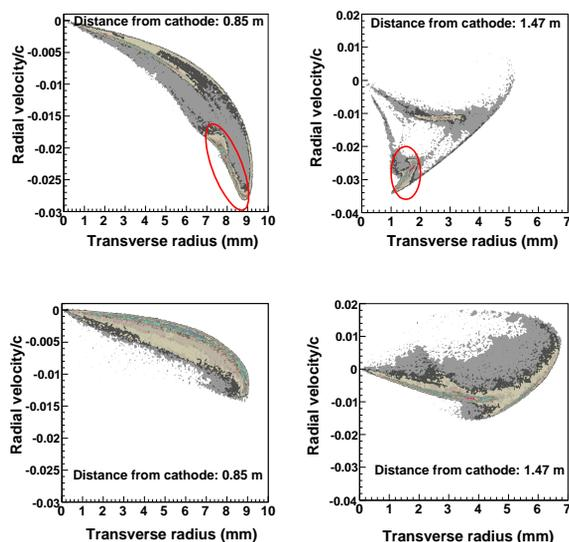
Figure 6: Slices of the phase space showing the radial velocity vs. the distance from the beam axis when the initial beam radius is 2 mm (upper plots) and 4 mm (bottom plots). For each case the plots correspond to two z-locations: upstream and downstream of the first SRF cavity. The red marker shows the location of the particles that generate the halo further downstream of the first SRF cavity.
