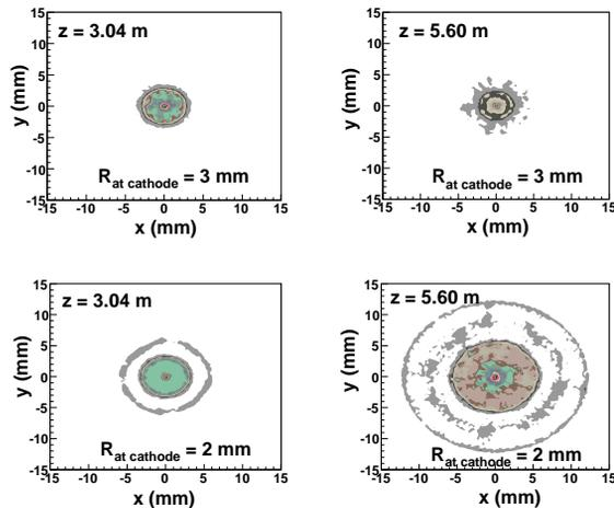
Figure 3: Transverse slices of the phase space at the entrance in the third accelerating cavity (left) and at the exit from the photoinjector (right). The radius of the beam at cathode was 3 mm (upper plots) and 2 mm (bottom plots).
