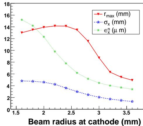
Figure 4: The distance between the outermost particle and the beam axis ( $r_{max}$ ), the radius of the beam (rms), and the normalized transverse emittance as functions of the beam radius at cathode.
