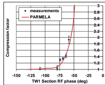
Figure 2: First velocity bunching: compression factor. Comparison between measurements and simulations.
