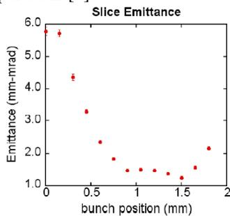
Figure 1: Slice emittance measurements. The slice length has been set to 150  $\mu$  i.e. about 0.5 ps.
