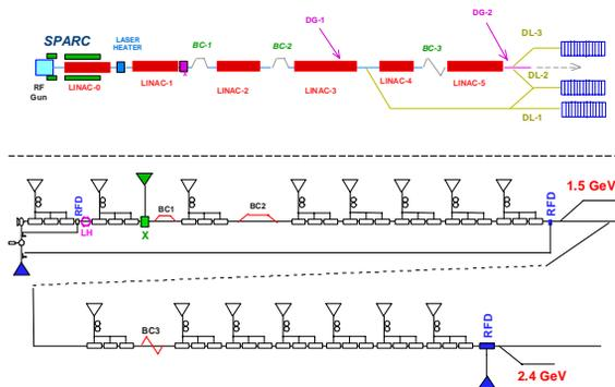
Figure 5: Layout and RF system of SPARX.
