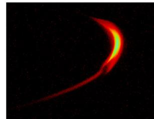
Figure 3: Imaging of long. phase space with the RFD. Beam energy: hor. axis; beam phase vert. axis.
