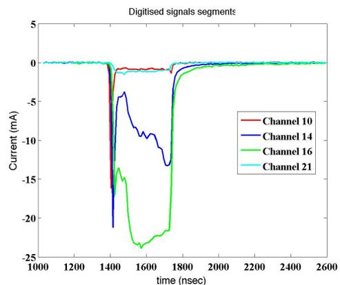
Figure 2: Typical digitised signals from segmented dump.
