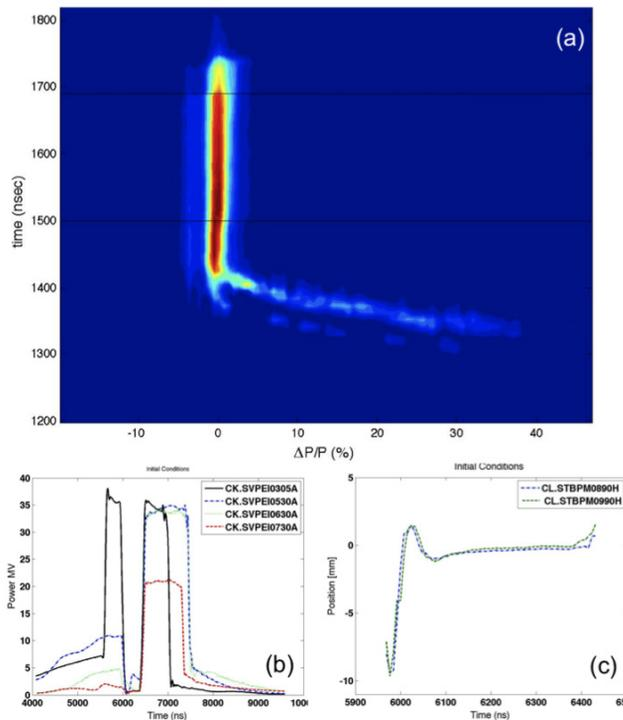
Figure 7: Initial Conditions. (a) The time resolved energy profile as measured with the segmented dump on spectrometer 10. (b) Output rf power measured from the accelerating structures (c) The horizontal position as measured with a beam position monitor on girders 8 and 9.
