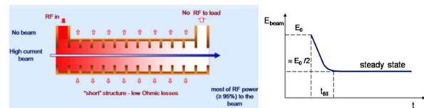
Figure 6: A schematic of the full beam loading concept.
