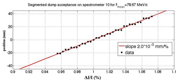
Figure 4: The horizontal dimension  $\pm 48$  mm for the segmented dump in spectrometer 10 corresponds to an energy spread acceptance of about 10%.
