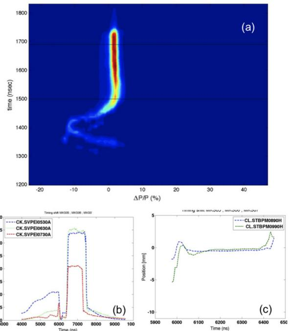
Figure 8: Delay arrival of rf from MKS05 by 400 ns; MKS06 by 550 ns and MKS07 by 250 ns with respect to the nominal conditions in Fig. 7. (a) The time resolved energy profile as measured with the segmented dump on spectrometer 10. (b) The output power measured from the accelerating structures. (c) The horizontal position as measured with a beam position monitor on girders 8 and 9.
