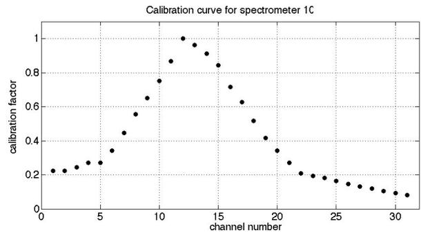
Figure 5: The calibration curve for the response of each segment of the segmented dump on spectrometer 10.
