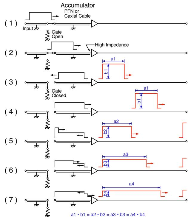
Figure 1: Principle of integrator circuit.
