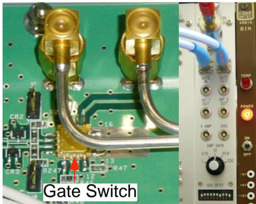
Figure 3: Gate switch on a base plate (left) and an exterior of developed integrator circuit (right).
