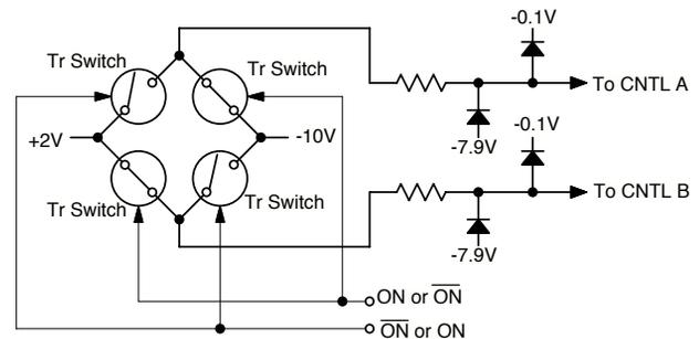
Figure 4: Block diagram of the circuit to generate control voltages for SW-283-PIN.
