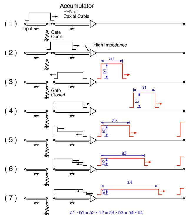
Figure 1: Principle of integrator circuit.
