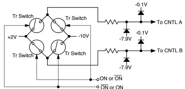
Figure 4: Block diagram of the circuit to generate control voltages for SW-283-PIN.
