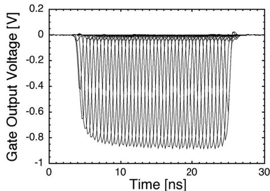
Figure 5: Superimposed 61 waveforms after passing gate switch.
