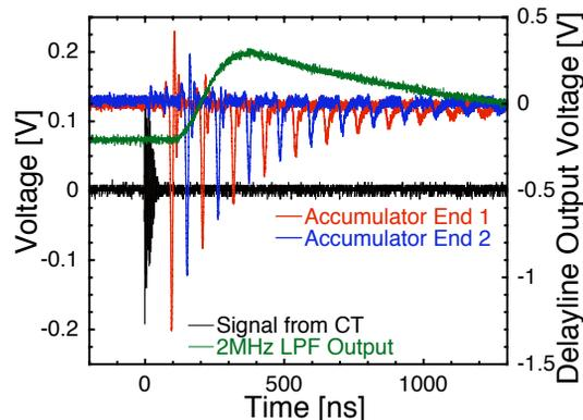
Figure 6: Voltages that appear at both ends of accumulator.
