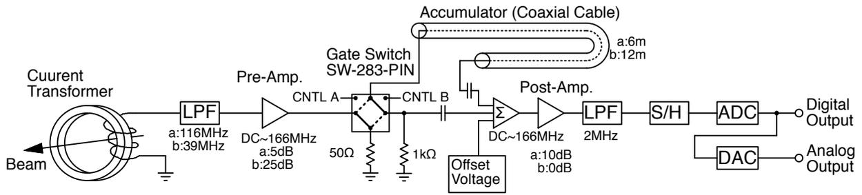
Figure 2: Block diagram of developed integrator circuit.
