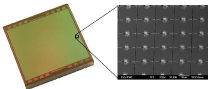
Figure 4: MMA with Enlargement of pixel structure[10].
