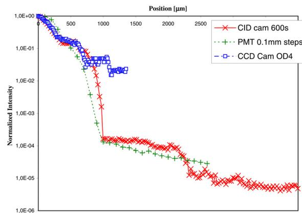
Figure 2: Beam profile of CCD (blue), CID (red) and PMT (green) [5].
