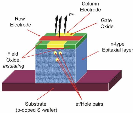
Figure 1: Layout CID pixel.
