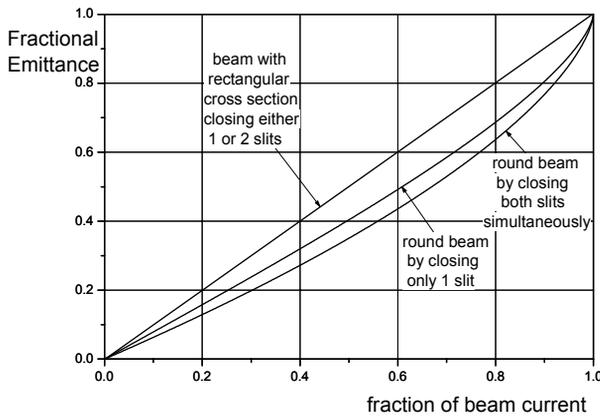
Figure 3: Theoretical variation of the fractional emittance on the transmitted current fraction for beams of uniform current density and rectangular or round cross section and for the cases of closing 1 slit only or 2 slits simultaneously.
