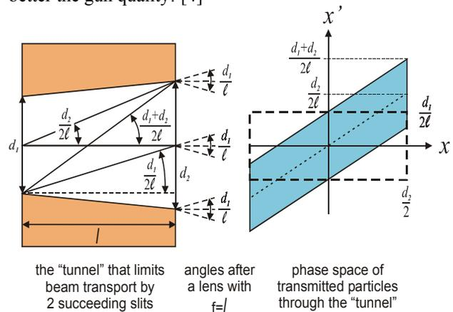
Figure 1: Definition of the tunnel emittance, showing how angles are defined by slit widths and the distance of the two apertures (left panel) and how this translates to the 2D phase space (right panel).
