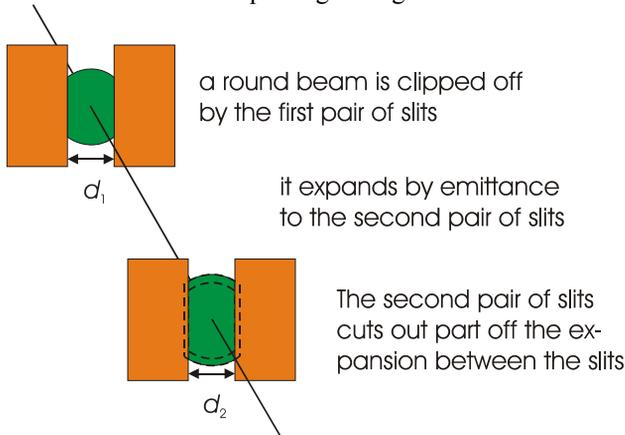
Figure 2: Measurement of full and fractional tunnel emittance by a pair of adjustable slits. For non-axisymmetric beams 2 pairs of slits in x and y-directions are needed. The transmitted beam then has a well defined, tailored emittance.
