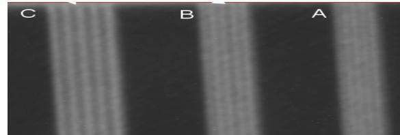
Figure 2: X-ray figure of a MTF chart.
