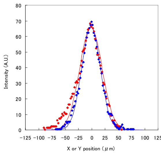
Figure 1: X-ray source distribution on the anticathode.
