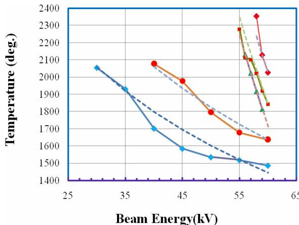
Figure 6: Energy dependence of the temperature at the irradiated area of the rotating antitarget.
