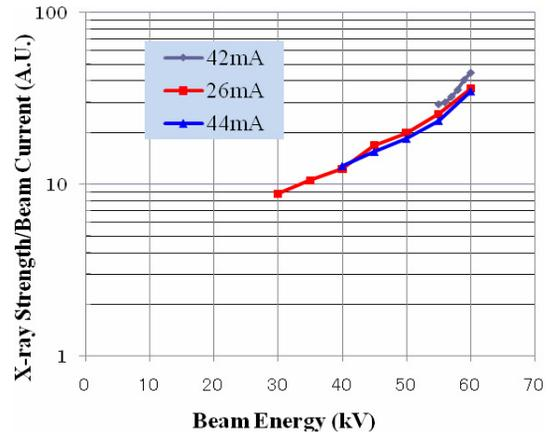
Figure 7: Energy dependence of X-ray strength.
