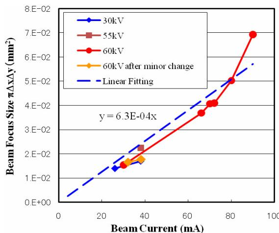
Figure 4: Current dependence of focus size.
