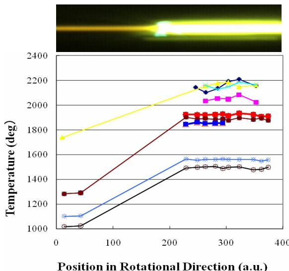
Figure 5: Temperature distribution of the target in rotational direction before and after irradiation.
