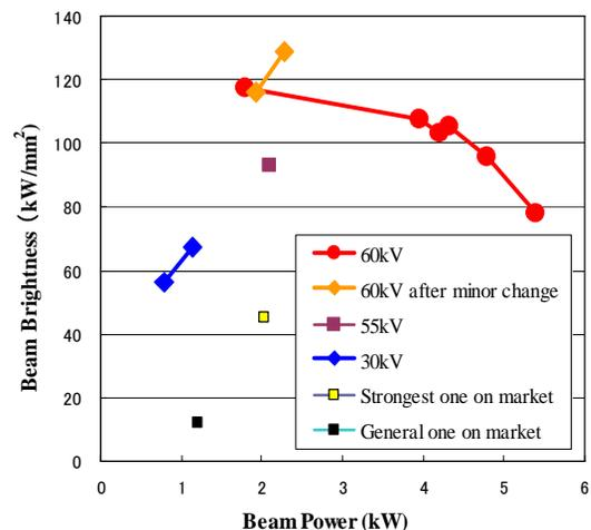
Figure 3: Beam power dependence of brightness.
