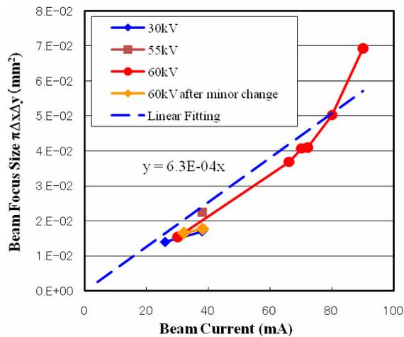
Figure 4: Current dependence of focus size.
