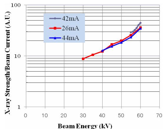
Figure 7: Energy dependence of X-ray strength.
