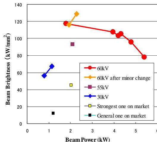
Figure 3: Beam power dependence of brightness.
