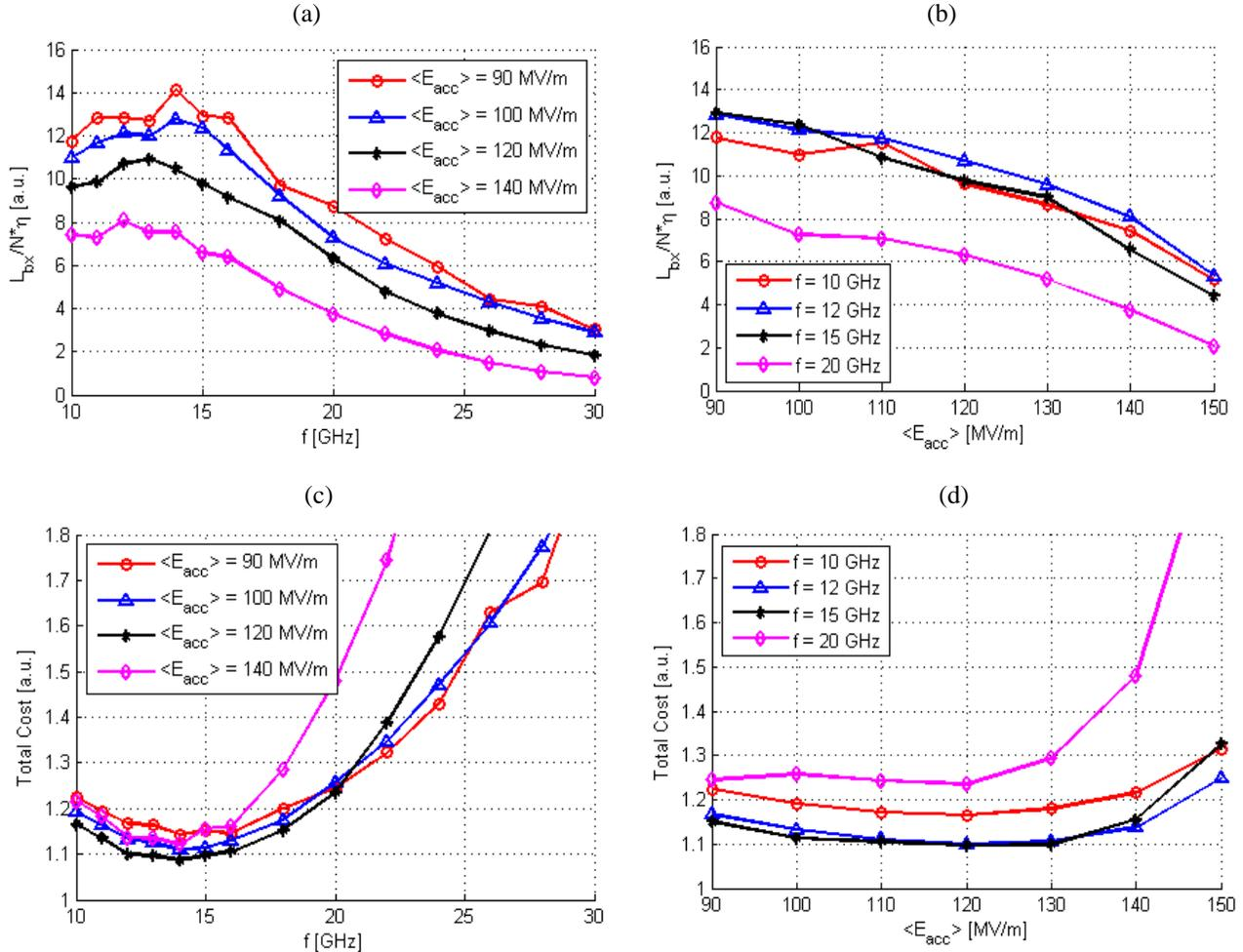
Figure 1: The results of optimization are presented both FoM on the top and for the total cost at the bottom.
