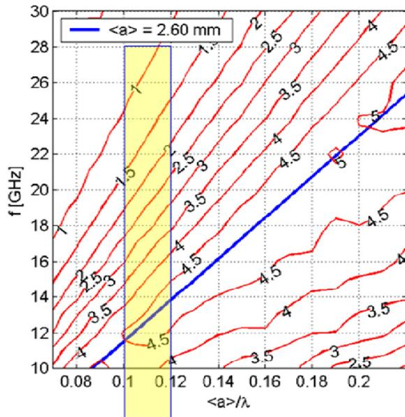
Figure 2: Lines of constant luminosity per bunch crossing normalized to the bunch population are plotted versus frequency and average ratio of aperture to the wavelength.
