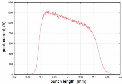
Figure 8: Peak current distribution at the end of the spreader obtained in tracking of 1B macroparticels through the entire machine beginning from the end of the injector using IMPACT.
