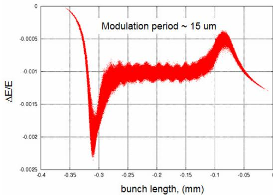
Figure 9: Longitudinal phase space at the end of the spreader obtained in tracking of 1B macroparticels through the entire machine beginning from the end of the injector using IMPACT.
