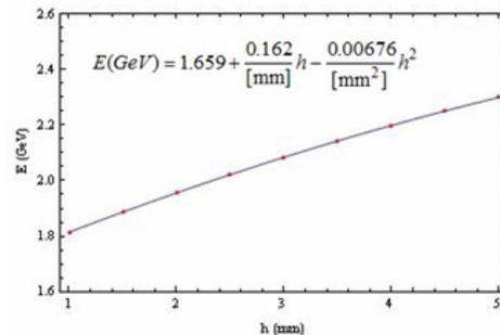
Figure 2: The electron beam energy that supports production of the x-rays within the range of wave lengths from 1 nm to 1.5 nm as a function of the size of the beam-stay-clear gap *h* in APPLE-II undulator.
