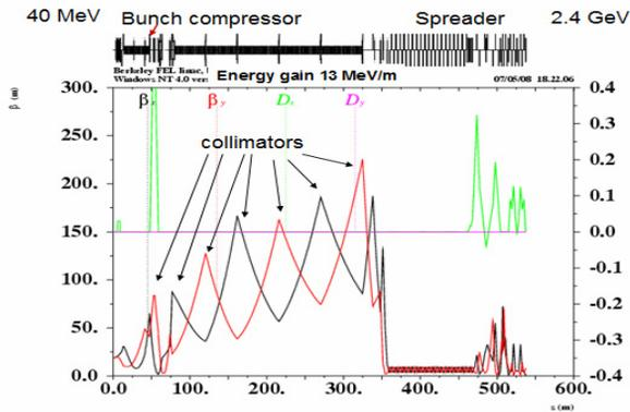
Figure 4: Linac lattice beginning from the end of the injector.
