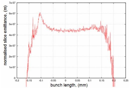
Figure 11: Normalized slice emittance at the end of the spreader obtained in tracking of 1B macroparticels through the entire machine beginning from the end of the injector using IMPACT.
