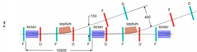
Figure 6: Beam take-off section of the spreader. Only two out of ten neighboring beamlines are shown.
