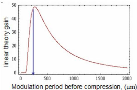
Figure 10: Gain of the microbunching instability. Arrow indicates modulation period obtained in macroparticle tracking (after accounting for a compression factor).
