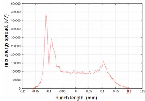
Figure 12: Slice rms energy spread at the end of the spreader obtained in tracking of 1B macroparticels through the entire machine beginning from the end of the injector using IMPACT.
