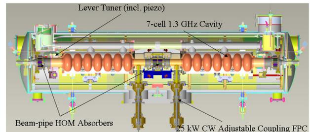
Figure 4: DICC Collaboration Cryomodule.
