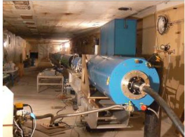
Figure 2: The injector of electrons with buncher, short accelerating section and four long accelerating section.
