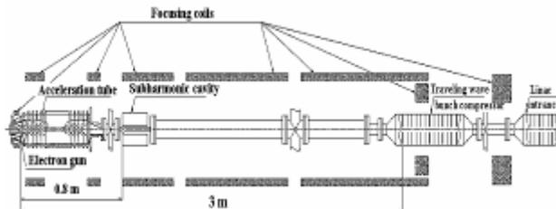
Figure 1: Injector layout.
