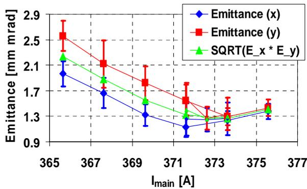
Figure 1: Transverse normalized projected emittance for different main solenoid currents at a bunch charge of 1 nC. Relevant machine parameters are given in the text. The numbers represent 100% RMS values.
