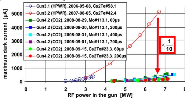
Figure 4: Maximum dark current for different gun cavities treated with different cleaning techniques.
