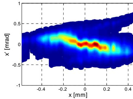
Figure 2: Detailed sampling of the horizontal phase space at the smallest emittance shown in Fig. 1 ( $I_{main} = 372.5$  A).
