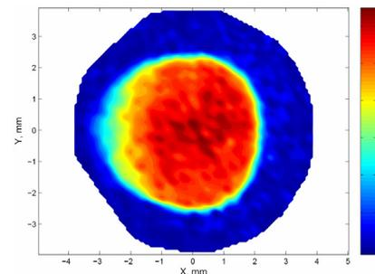
Figure 7: Quantum efficiency map of Cs<sub>2</sub>Te cathode #23.3. The colour code gives relative information only.
