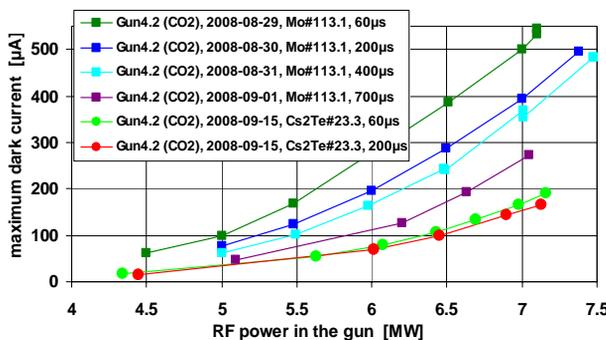
Figure 5: Maximum dark current for different RF pulse lengths and cathodes, ordered in sequence of data taking.
