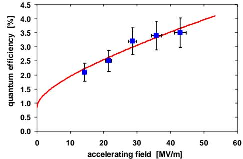
Figure 6: Quantum efficiency of Cs<sub>2</sub>Te cathode #23.3 as a function of the accelerating field at the photo cathode.
