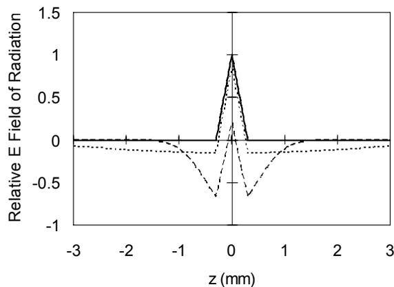
Figure 2: Pulse shape of the electric field of the coherent synchrotron radiation obtained by calculation for the isosceles triangular electron bunch at a FWHM length of 1 ps. No suppression (solid line) and suppression of radiation at wavelengths longer than a cutoff wavelength of 1 (dashed line) and 5 (dotted line) mm have been assumed.
