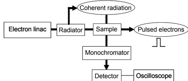
Figure 3: Schematic diagram of the pump-probe experimental setup.
