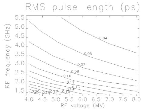
Figure 5: Minimum pulse length as a function of rf frequency and voltage.
