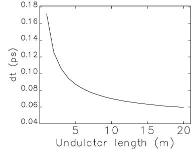
Figure 3: Minimum pulse length dependence on the undulator length for  $V=6$  MV,  $\omega=2\pi\cdot 2.8$  GHz, and  $\lambda=1.2$  Å.
