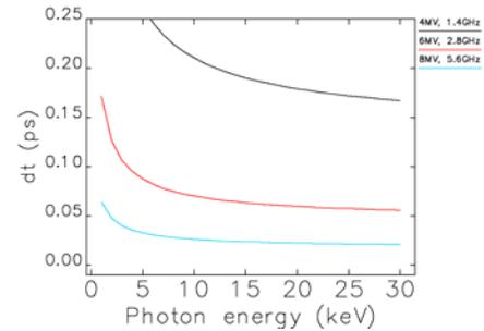
Figure 4: Minimum pulse length dependence on the photon energy for different rf voltages and frequencies.
