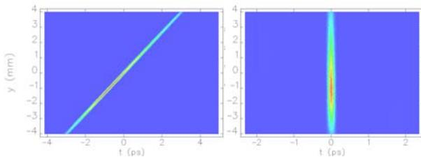
Figure 6: Photon pulse shapes before (left) and after (right) compression.
