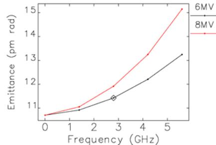
Figure 8: Vertical beam emittance after the second deflecting cavity for different rf frequencies and voltages. A diamond symbol shows the point corresponding to the parameters in Table 1.
