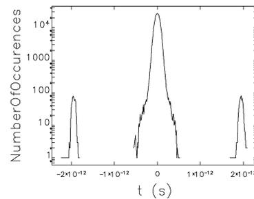
Figure 7: Photon pulse profile. The rms pulse length is 62 fs. Small peaks at around  $\pm 2$  ps are produced by the second-harmonic radiation.
