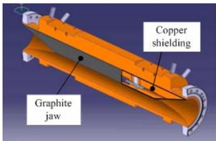
Figure 5: Final bi-material jaw of the TCC.
