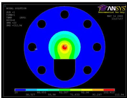
Figure 3: Temperature distribution in TCC active part during dump operation.
