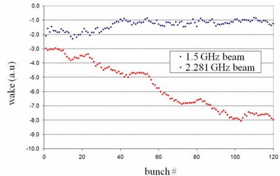
Figure 4: The wake seen by different bunches. The value for bunches with a spacing of 1.5 GHz (real operation) is constant. An artificial bunch frequency of 2.281 GHz served to validate the method; in this case the build-up is evident.
