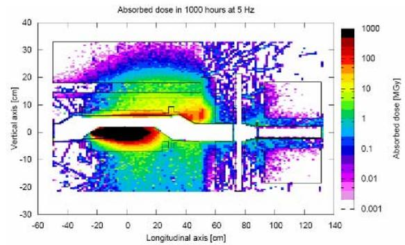
Figure 7: Absorbed dose in the TCC and downstream quadrupole after internal and external shielding.
