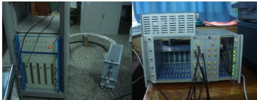
Figure 8: Pictures of RF amplifier under test.
