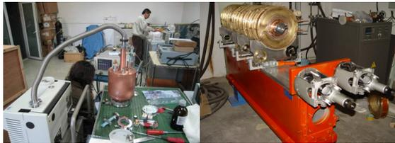
Figure 7: SHB cavity tuning (left) and system pre-installation (right).
