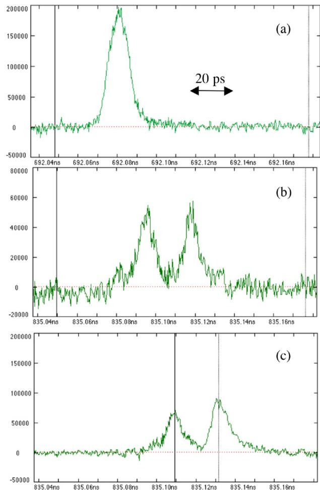
Figure 4: Bunch structure measured with streak-camera systems utilizing OTR located before and after the 180-degree arc section: (a) observed before the arc, (b) and (c) after the arc. (a) and (b) are the cases for a charge of 1 nC, while (c) is for 2 nC.
