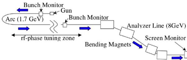
Figure 2: Schematic view of the experimental setup. The longitudinal phase space of the single-bunched electron beam is diagnosed by two methods: one with the bunch monitors before and after the arc, the other utilizing the 8-GeV energy analyzer line located at the end of the linac.
