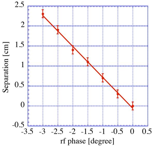
Figure 5: Energy separation of the two microbunches as a function of the rf phases. The data points are fitted with the function  $x$  given in the text.
