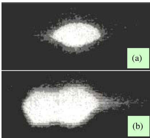
Figure 3: Energy profiles observed on the screen monitor at large dispersions: (a) for the single bunch in optimum rf acceleration phases and (b) for those split into two clusters in non-optimum rf phases.
