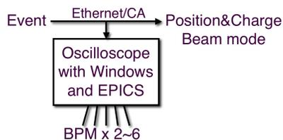
Figure 4: 24 oscilloscopes are installed to read 100 BPMs in 50 Hz distinguishing the beam modes.
