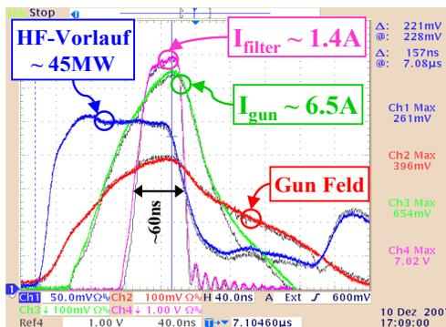
Figure 3: Scope traces of RF-gun pulses. At very high forward power of 45 MW over 160 ns filtered beam currents of 1.4 A are achieved
