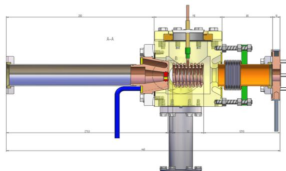
Figure 2: CAD model of the modified positron converter. In comparison to the old design all movable parts were eliminated and there are no more braze joints of water filled parts in vacuum.
