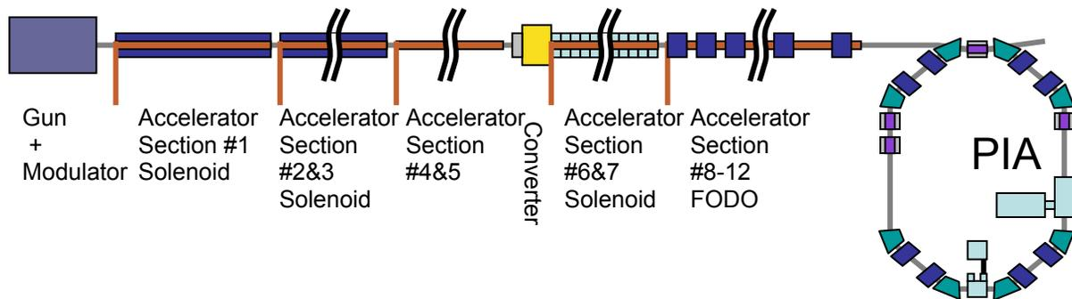
Figure 1: Schematic layout of the Linac II at DESY. The 6 A primary beam is produced in a 120 kV pulsed DC gun and directed onto a converter target at approximately 400 MeV. The secondary beam is accelerated to 450 MeV and injected into the Positron Intensity Accumulator (PIA).
