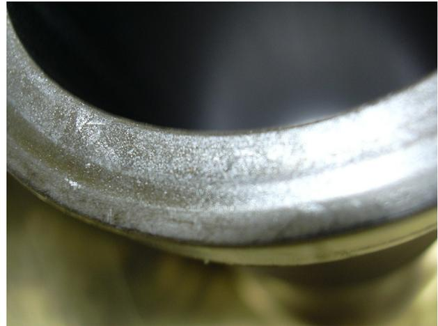
Figure 6: Picture of the cavity flange displaying an obvious score mark.
