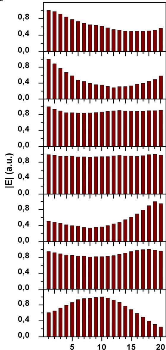
Figure 4: Measured field flatness of six cavities being in operation for some 10 years. Some cavities display a heavily distorted field profile that could be restored during the tuning procedure.
