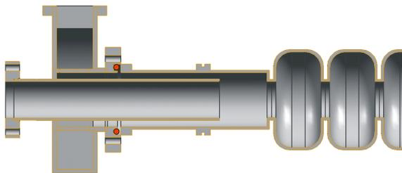
Figure 5: Cross section of the coupler to cavity transition. The HELICOFLEX® gasket used is marked red.
