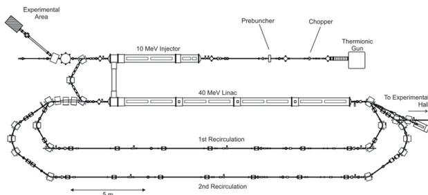
Figure 1: Floor plan of the S-DALINAC.
