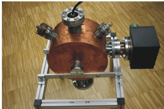
Figure 3: 500 MHz prebuncher.
