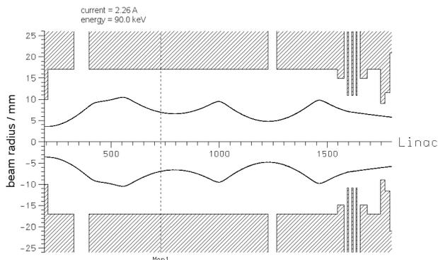
Figure 7: Simulation of a 2 A beam propagating through the beam guiding elements based on the paraxial equations.
