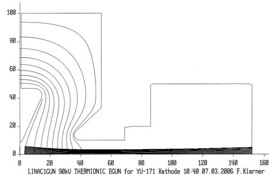
Figure 2: Gun geometry  $r$  vs.  $z$  in mm with equipotential lines and space charge limited electron rays calculated with EGUN for an anode voltage of 90 kV.
