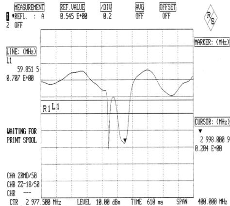
Figure 6: Plot of the reflected power against the RF frequency. The plot shows the passband of the structure.
