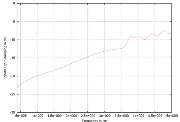
Figure 9: Measurements of the bandwidth of the wall current monitor. The results give an estimate of the bandwidth of the monitor. It appears, that the monitor will be useable for a range up to 3 – 3.5 GHz.
