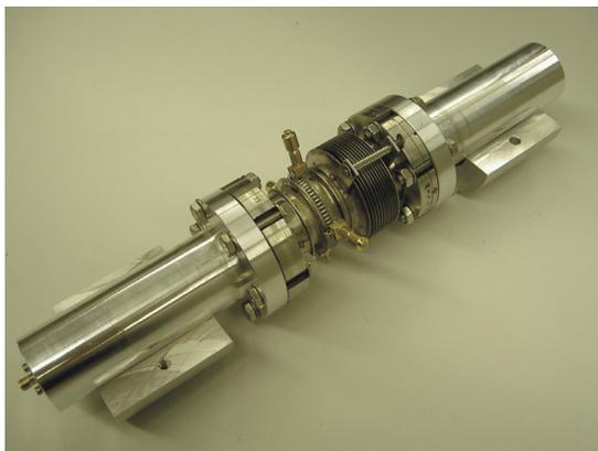
Figure 8: Wall current monitor with a bandwidth of 3 GHz, mounted on a special measurement setup to determine the bandwidth.
