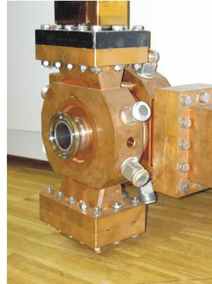
Figure 5: The travelling wave buncher with a view of the exit of the structure. On top a waterload is flanged. On the right hand side is the input of the accelerating RF.
