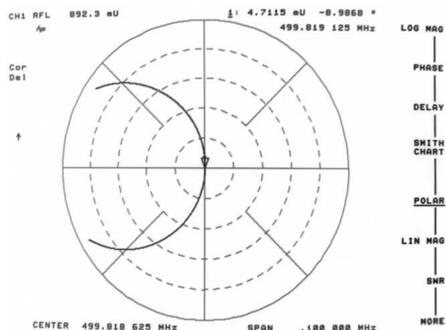
Figure 4: Polar plot of the complex reflection factor close to the first resonance of the prebuncher.
