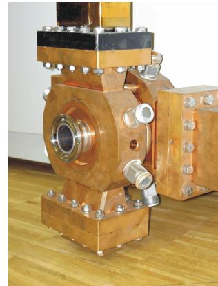
Figure 5: The travelling wave buncher with a view of the exit of the structure. On top a waterload is flanged. On the right hand side is the input of the accelerating RF.
