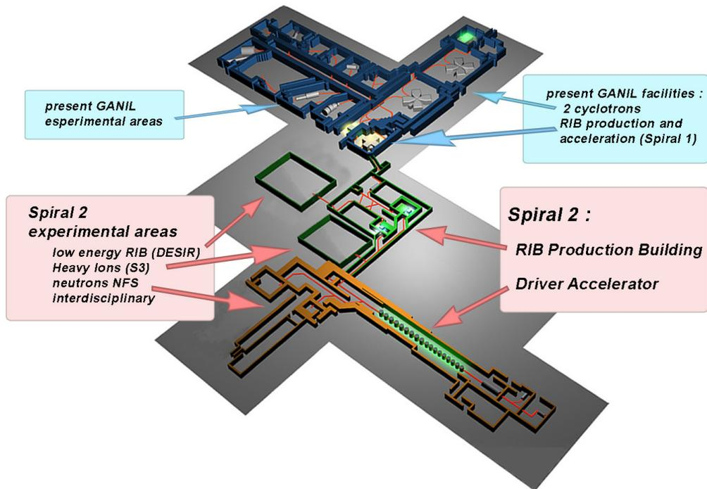
Figure 1: Present facilities at GANIL laboratory and new buildings for SPIRAL 2 Driver Accelerator and associated Experimental Areas.
