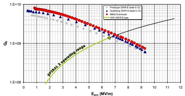
Figure 7: Accelerating gradient performances of  $\beta=0.12$  QWR ( 2 prototypes and first of serial production).
